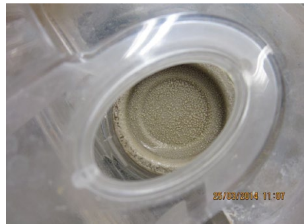
Figure 1: Respiratory device retrieved from case with biofilm on the internal filter
